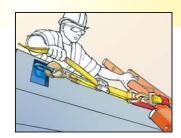
TIGHTEN BELT BY PULLING YELLOW ADJUSTING BELT
